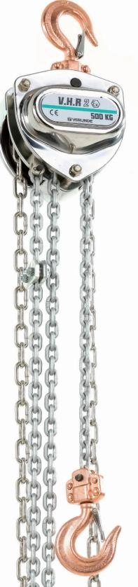
Manual trolleys and hand chain blocks designed to be used in explosive atmospheres do not have to comply with specific standards. However, the use of this type of lifting equipment of its very nature could lead to sparks (creation of particles by friction). To deal with this problem, VERLINDE's manual trolleys and hand chain blocks are available in ATEX version. Marking : Ex 11 2 Gc IICT4.
